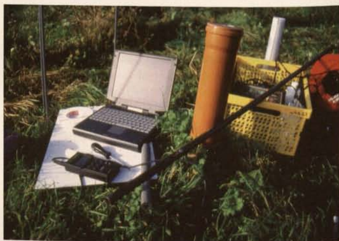
Fig. 7. Nydam Mose: Analytical devices with special designed micro-electrode devices (i.e. tube in front) to measure the oxygen levels respectively anoxic areas in the sediments of the excavation field.
