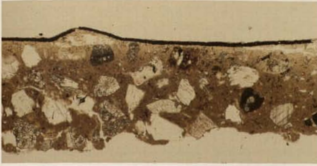
Fig. 5a. Padua, Scrovegni-Chapel: Stratigraphic section observed at transmitted light, parallel nicols, ob. 2.5x. Gypsum crystallization is visible under the pictorial layer.
