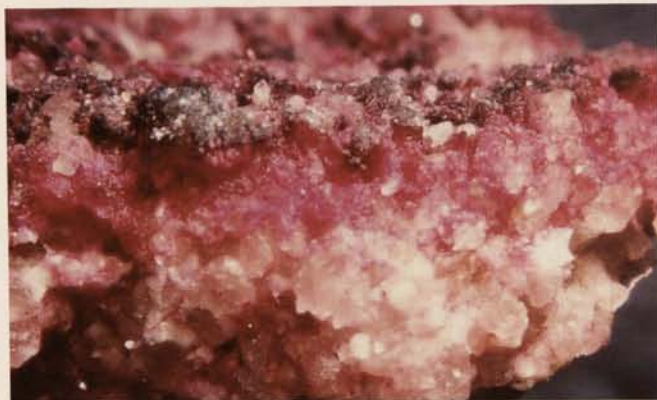
Fig. 2. Pommersfelden, Castle Weissenstein, detail: Microbial biofilm penetrating into the pore system of a natural stone (i.e. Burgsandstein) as visualized by red PAS-staining.
